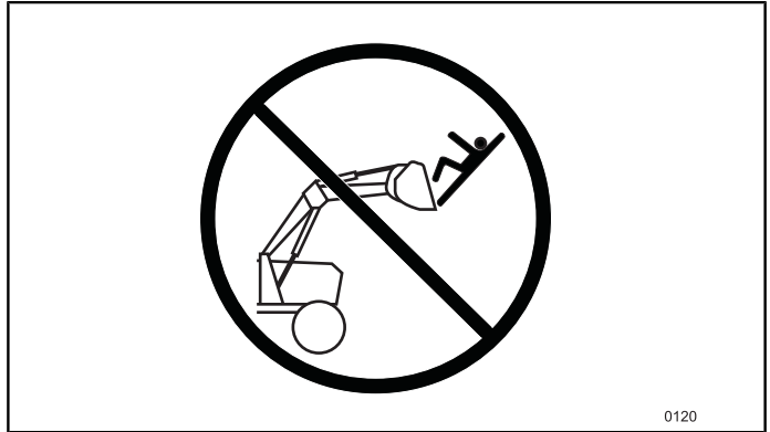
Fig.7 Do NOT use the loader or the attachment as a working platform.
