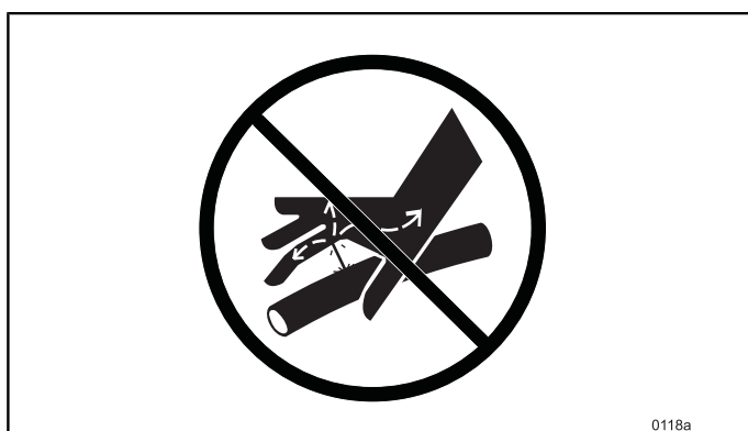
Fig.13 NEVER use fingers or hands for leakage detection.
