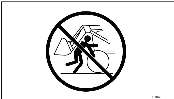
Fig.30 Never stand between the front of the tractor and the loader's cross tubes.
