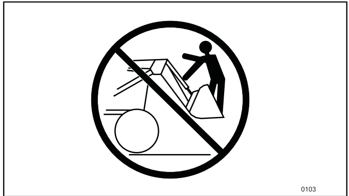
Fig.8 Do NOT use the loader or attachment to lift or transport people.
