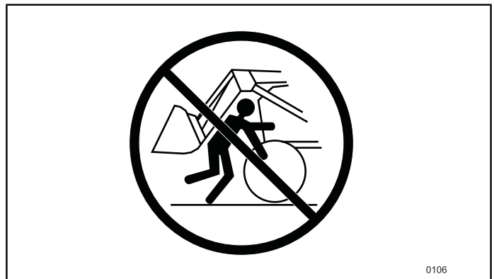
Fig.14 Never stand between the front of the tractor and the loader's cross tubes.
