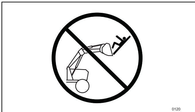
Fig.9 Do NOT use the loader or the attachment as a working platform.
