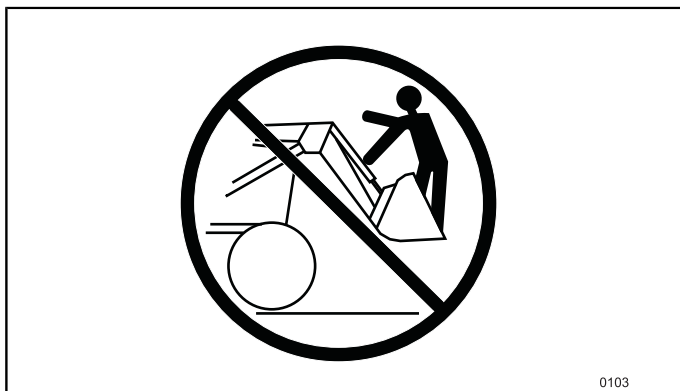
Fig.10 Do NOT use the loader or attachment to lift or transport people.
