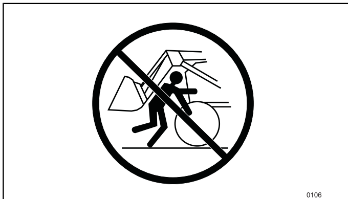
Fig.26 Never stand between the front of the tractor and the loader's cross tubes.
