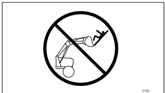
Fig.7 Do NOT use the loader or the attachment as a working platform.
