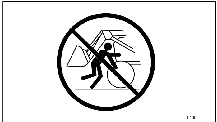
Fig.12 Never stand between the front of the tractor and the loader's cross tubes.
