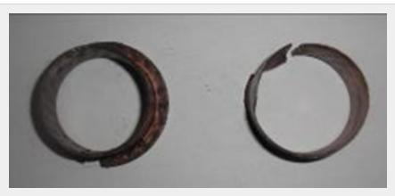
Figure 7.30: Example picture of plain bearing. New bearing to the left, and worn out/defect bearing to the right.
