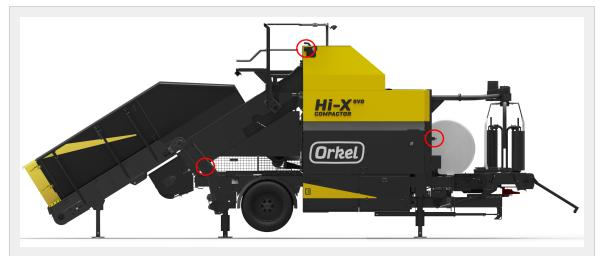
Figure 2.1: Red circles indicates emergency stop locations. Two more buttons are located on the opposite side, ground level.
