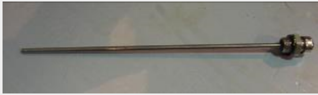
Figure 7.31 : Dipstick with max and min level indicators
