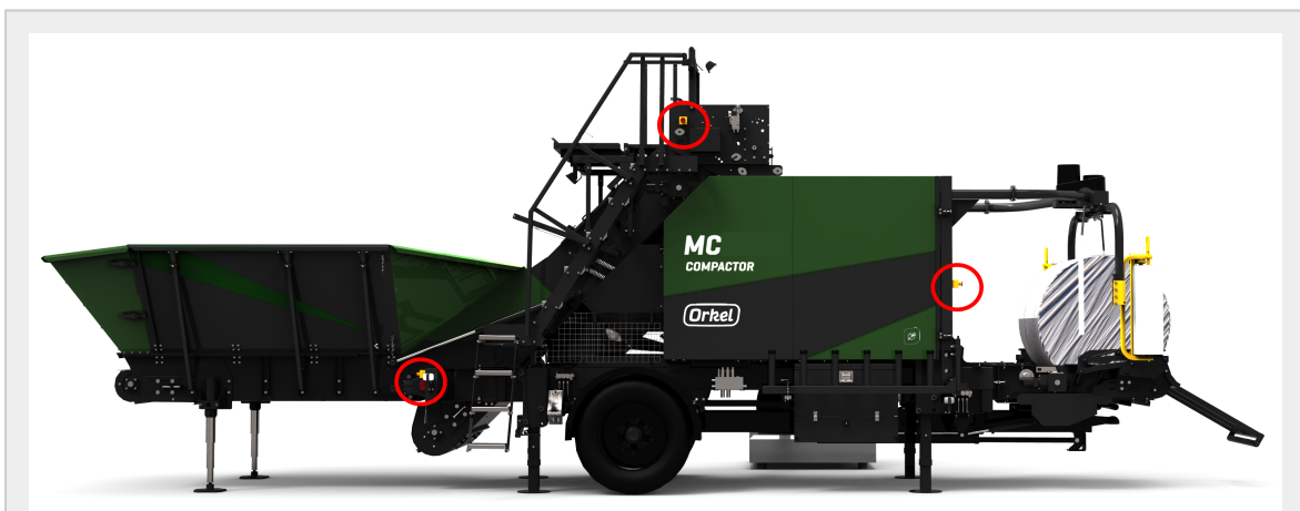
Figure 2.1 : Red circles indicates emergency stop locations. Two more buttons are located on the opposite side, ground level.
