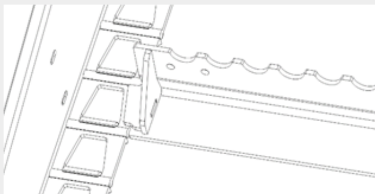
Figure 7.5 : Elevator conveyor chain
