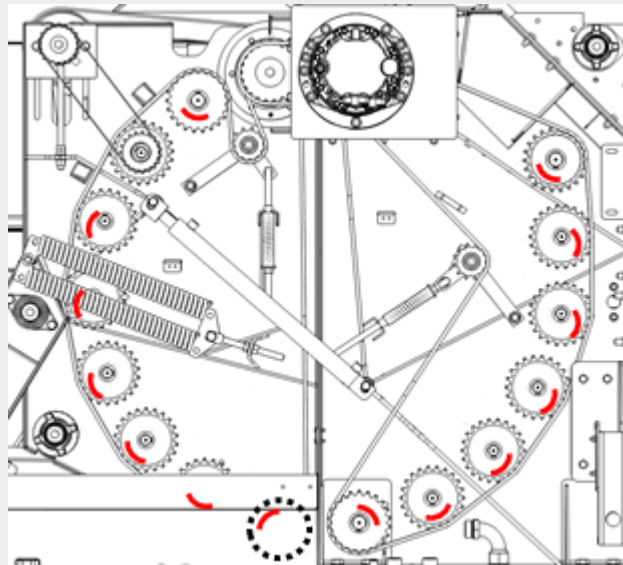
Figure 7.27 : Check for play in the bushings. Red markings indicate areas on the bushings.
