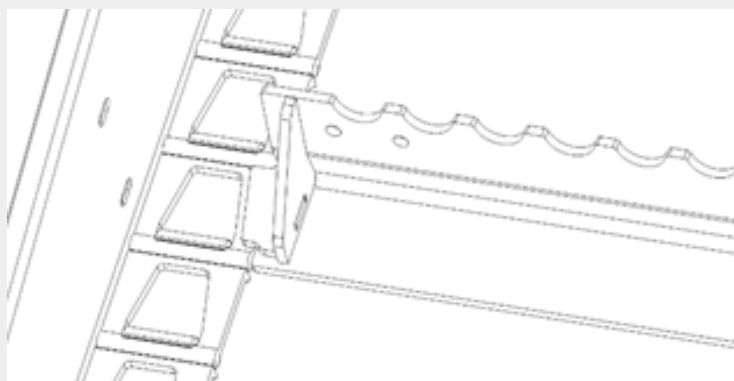
Figure 7.12 : Elevator conveyor chain
