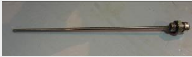
Figure 7.36 : Dipstick with max and min level indicators
