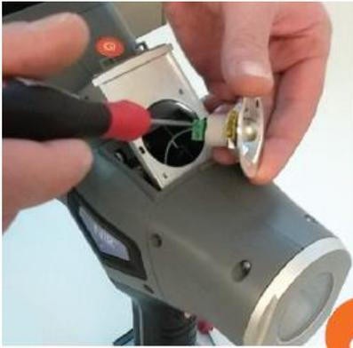
CAREFULLY disconnect the cable from the lamp.
