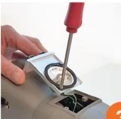
Unscrew the seal support of the lamp
