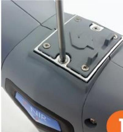
Unscrew the two screws of the lamp cover on top of X-NIR™
