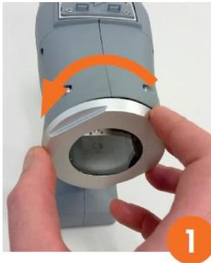
Turning the reading glass counterclockwise
