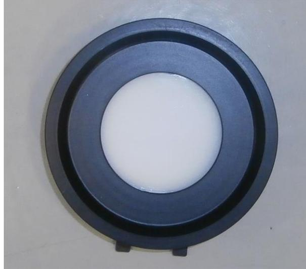
**CHECK CELL** ← particular sample in acetal resin for the X-NIR™ tests.
