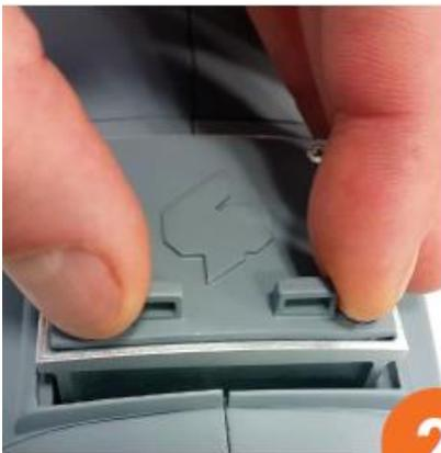
CAREFULLY pull out the lamp by lifting the two hooks on top
