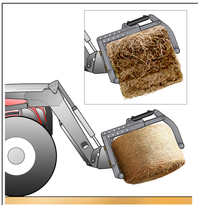
Fig.25 Transport the material as low as possible
