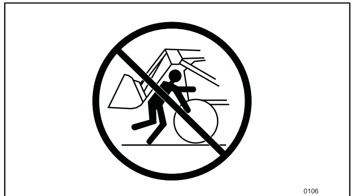
Fig.13 Never stand between the front of the tractor and the loader's cross tubes.
