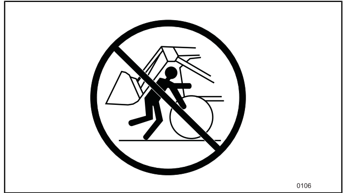
Fig.27 Never stand between the front of the tractor and the loader's cross tubes.
