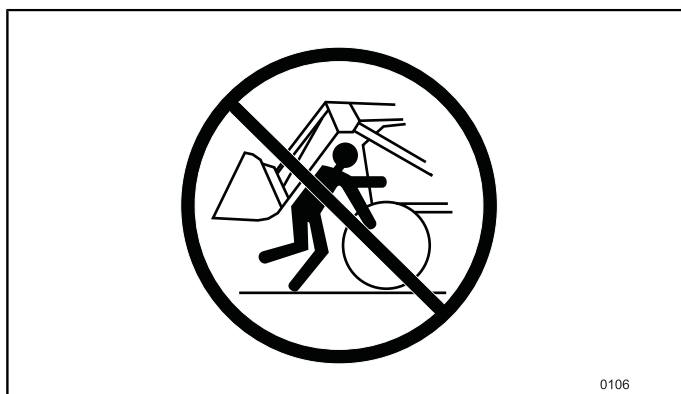
Fig.20 Check carefully that there is no risk of collision between loader and implement.
