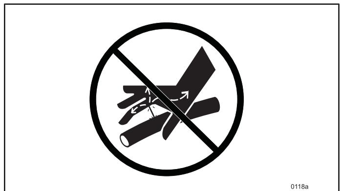
Fig.14 NEVER use fingers or hands for leakage detection.
